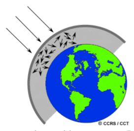
**Rayleigh scattering** occurs when particles are very small compared to the wavelength of the radiation. These could be particles such as small specks of dust or nitrogen and oxygenmolecules. Rayleigh scattering causes shorter wavelengths of
