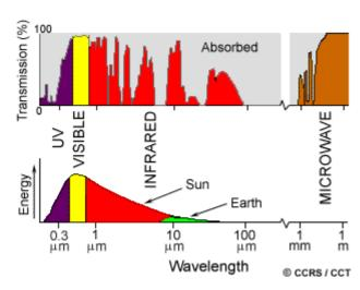
Because these gases absorb electromagnetic energy in very specific regions of the spectrum, they influence where (in the spectrum) we can "look" for remote sensing purposes. Those areas of the spectrum which are not severely influenced by atmospheric absorption and thus, are useful to remote sensors, are called **atmospheric** windows. By comparing the characteristics of the two most common energy/radiation sources (the sun and the earth) with the
